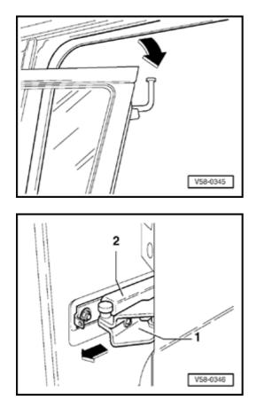
Lower sliding door at front until upper roller guide can be removed from guide rail.
