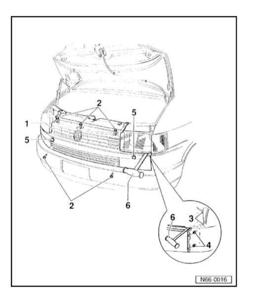
Radiator grille with trim frame, removing and installing (from 01.96)
