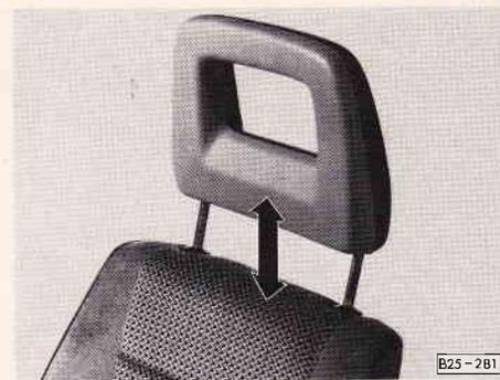
■ For height adjustment grasp head restraint with both hands and pull up or push down.
