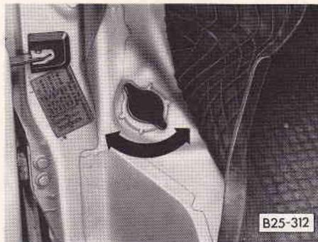
The filler cap is located at the left side of the driver's footwell.
