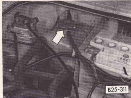
Expansion tank Diesel engine
