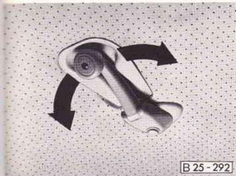
**To open** pull crank handle out of recess and turn counter-clockwise.
