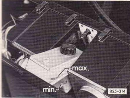
The brake fluid reservoir is located under the instrument cluster in the dashboard panel.
