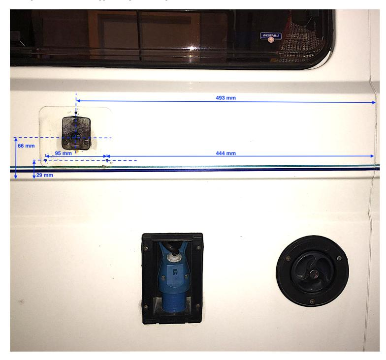
Drilling plans valid in Europe, for vehicles chassis F (1985) to chassis N (1992)
