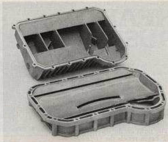
We mustn't forget the bottom end—a baffled and finned alloy deep sump holds the oil in place. Above, a windage tray keeps oil aeration to a minimum and reduces drag on the crankshaft.
