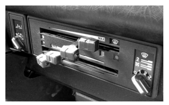
**TOP LEVER:** The "defrost" lever. This lever operates a cable that moves flaps in the air distribution box, increasing or decreasing fresh airflow to the windshield and front door windows. The air flows via the four air ducts on the top surface of the dashboard (numbered "1" and "2" in your owner's manual, page 45). The air controlled by this lever can be either cool or heated air, depending on where the second lever is positioned.
