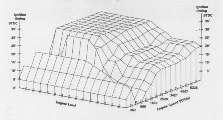
The map controlled ignition system operates on the principle of a timing map which is programmed into the E.C.U. Information on engine load, speed and coolant temperature are provided to the E.C.U. in the form of voltage signals. In the E.C.U. these signals are processed so that the ignition coil is controlled via terminal #1 in accordance with the programmed ignition map. The separate ignition control unit and digital idle stabilizer used in the past have been eliminated.
