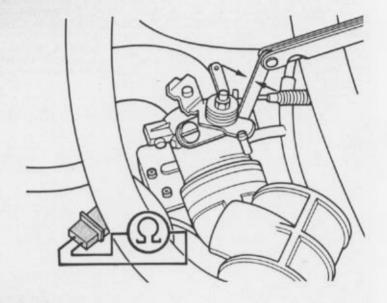
At point switch contacts close, Gap A must be between 0.05 - 0.10 mm (.002 - .004 in.)
