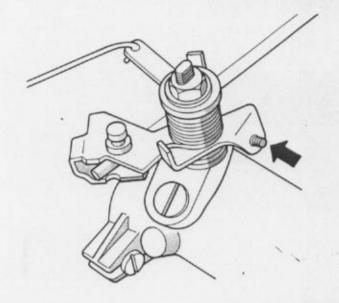
Note: Stop screw is set at factory and should not be moved. If screw position has been altered, check basic adjustment as follows:
