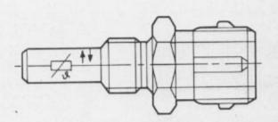
The coolant temperature sensor is a negative temperature coefficient resistor (NTC). The resistance signal it produces is used by the control unit to determine:
