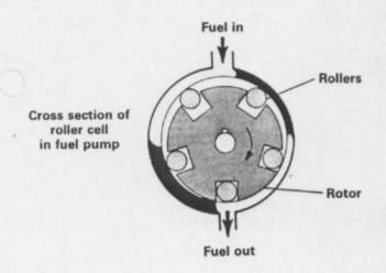
The fuel pump is a roller cell design. It is driven by a permanent magnet electric motor and is located near the fuel tank.
