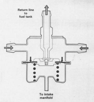
The system pressure regulator maintains a constant fuel pressure to all injectors by regulating the quantity of fuel returned to the fuel tank.
