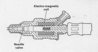
Digifant fuel injectors are electronically controlled on/off valves. A solenoid actuates a needle valve allowing fuel to be forced through the injector nozzle. All four injectors open at the same time and inject fuel directly into the intake manifold near the intake valve. Injection quantity is controlled by the amount of time the injectors stay open. Injector opening time is regulated by the E.C.U., based on inputs from the various engine sensors.
